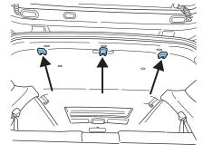
3. Clip the tether strap to the anchor as shown.
